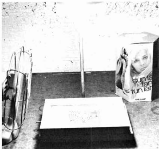
fig. 13. Circuit board is exposed to ultraviolet lamp for about 15 minutes. Fan keeps the photoresist from getting too hot.
